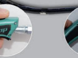
A distance remote control; advantage: a single hand to hold the tip and starting the machine.
